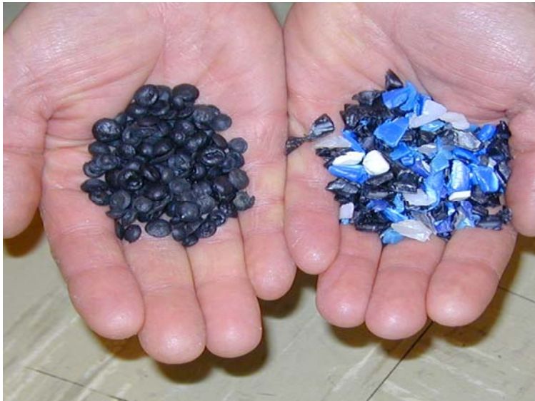
Figure 3. The two fuels consumed during air emissions testing, l to r, Korean LDPE pellets made from waste agricultural mulch film, and HDPE granulated barrels.
