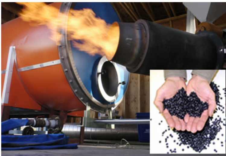
Figure 2. The GR Technologies, Inc. burner fueled on plastic pellets (inset) made from waste agricultural mulch
